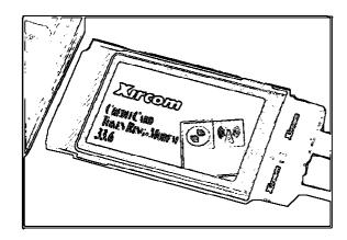
Combination 16/4 Token-Ring and high-speed 33.6 modem in a single PC Card
